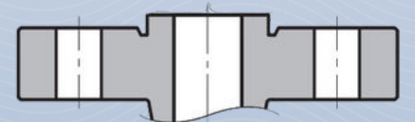
TYPE G AND H - O-RING SPIGOT AND O-RING GROOVE FACE
