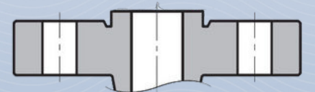
TYPE G AND H - O-RING SPIGOT AND O-RING GROOVE FACE
